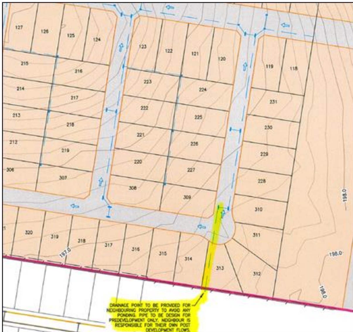
Figure 7: Stormwater flow from the south-east can be collected at this point and dispensed through the proposed development's road and drainage network.
